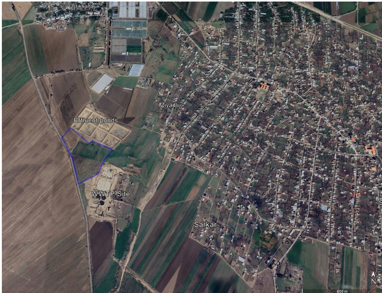
Figure 2. The sites of the WWTP and effluent ponds, and a proposed location of additional land (blue contour) that may be procured for sludge management, if agricultural re-use is not feasible
